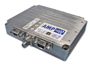
AMP's ET80 Series 7.7 cubic inch encrypted video/audio transmitters offer innovative features and high quality packaging and connectors. Like all E-Series products, ET80 models feature Micro-ViewLockII, or Micro-View/AudioLockII when equipped with audio, for secure video communications. A secondary encryption key may be programmed for maximum security.
